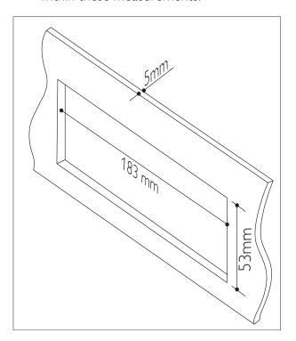
Install the sleeve into the dashboard and bend the tabs outward to fix the sleeve.
